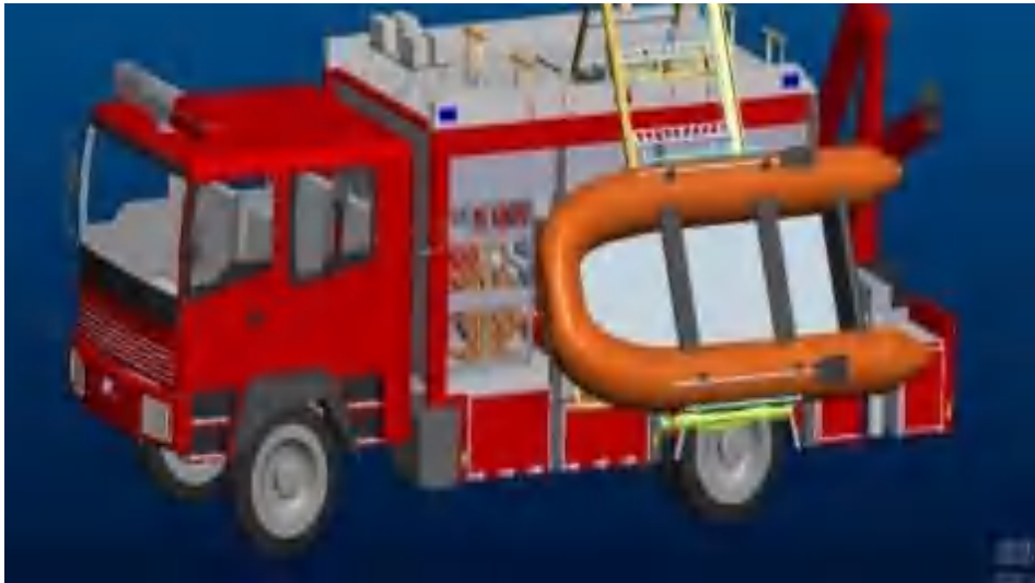
UNFOLD STATUS(EXTENDS OUTWARD BY ABOUT 2 METERS FROM THE ROOF OF APPARATUS)
