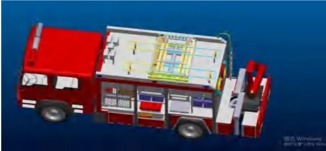
UNFOLD STATUS(EXTENDS OUTWARD BY ABOUT 2 METERS FROM THE ROOF OF APPARATUS)
